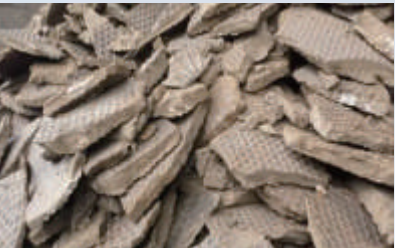
Raw Material Before Drying Moisture content 55% - 65%, blocky, with more crushed material after conveying
