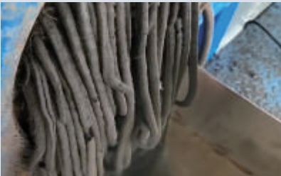
After Forming Material in strip form, compact and distinct, with less crushed material
