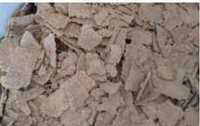
Raw material before drying Moisture content 40%, irregular flake - shaped, loose, with more crushed material
