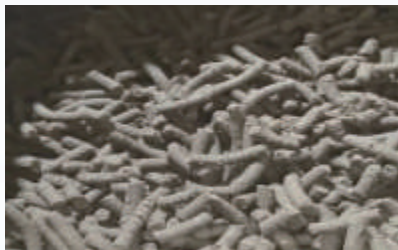
Product After Drying Moisture content 10%, uniform dryness of the finished product, with less crushed material
