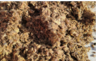
Raw material before drying Moisture content 60%, livestock bedding, irregular fibrous material
