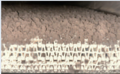
Product After Drying Moisture content 30%, uniform dryness of the finished product, with less crushed material
